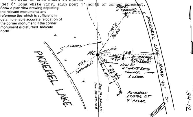
Describe any material discrepancy between the location of the corner as restored or reestablished and the location of that corner as previously restored or reestablished by distance and direction. Show the discrepancy on the plan view drawing under (d), above. Show the distances between the corner as previously restored or reestablished and (1) the corner as restored or reestablished, and (2) to at least 2 of the witness monuments shown on the drawing in (d), above.
