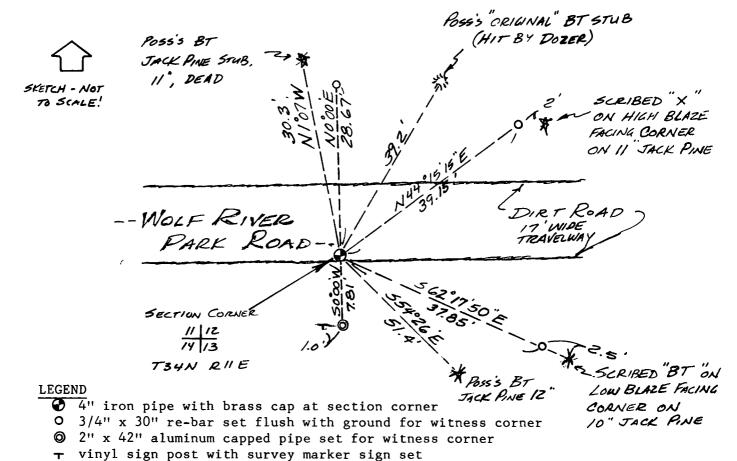
Distances to iron witness monuments measured with EDM. Compass bearing of N  $0^{\circ}00'$  E to north witness monument used as reference bearing for angles turned to the other witness's.
