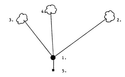
(e) Describe any material discrepancy between the location of the corner as restored or reestablished and the location of that corner as previously restored or reestablished by distance and direction. Show the discrepancy on the plan view drawing under (d), above. Show the distances between the corner as previously restored or reestablished and (1) the corner as restored or reestablished, and (2) to at least 2 of the witness monuments shown on the drawing in (d), above.
