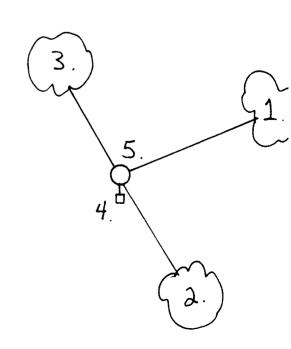
(e) Describe any material discrepancy between the location of the corner as restored or reestablished and the location of that corner as previously restored or reestablished by distance and direction. Show the discrepancy on the plan view drawing under (d), above. Show the distances between the corner as previously restored or reestablished and (1) the corner as restored or reestablished, and (2) to at least 2 of the witness monuments shown on the drawing in (d), above.
