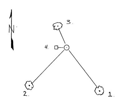
(e) Describe any material discrepancy between the location of the corner as restored or reestablished and the location of that corner as previously restored or reestablished by distance and direction. Show the discrepancy on the plan view drawing under (d), above. Show the distances between the corner as previously restored or reestablished and (1) the corner as restored or reestablished, and (2) to at least 2 of the witness monuments shown on the drawing in (d), above.
