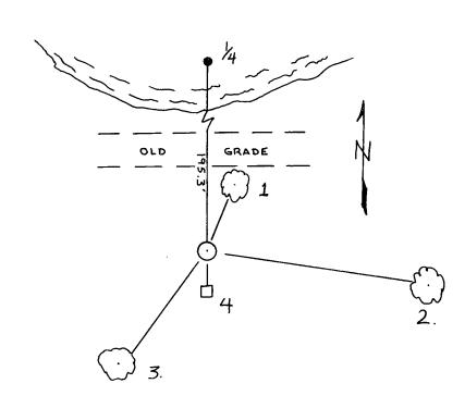
Describe any material discrepancy between the location of the corner as restored or reestablished and the location of that corner as previously restored or reestablished by distance and direction. Show the discrepancy on the plan view drawing under (d), above. Show the distances between the corner as previously restored or reestablished and (1) the corner as restored or reestablished, and (2) to at least 2 of the witness monuments shown on the drawing in (d), above.
