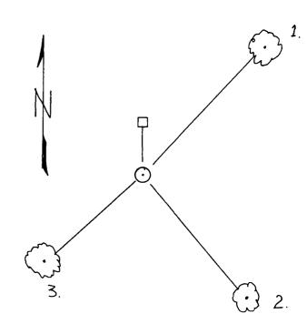
(e) Describe any material discrepancy between the location of the corner as restored or reestablished and the location of that corner as previously restored or reestablished by distance and direction. Show the discrepancy on the plan view drawing under (d), above. Show the distances between the corner as previously restored or reestablished and (1) the corner as restored or reestablished, and (2) to at least 2 of the witness monuments shown on the drawing in (d), above.
