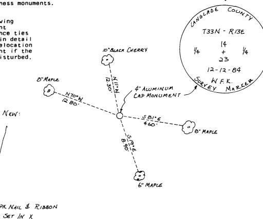
(e) Describe any material discrepancy between the location of the corner as restored or reestablished and the location of that corner as previously restored or reestablished by distance and direction. Show the discrepancy on the plan view drawing under (d), above. Show the distances between the corner as previously restored or reestablished and (1) the corner as restored or reestablished, and (2) to at least 2 of the witness monuments shown on the drawing in (d), above.
