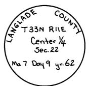
Dug eld peint out and reset pipe in same hele. Set brass cap welded into a 4 foot section of  $1\frac{1}{4}$ " pipe. Pipe extended 2 feet above ground and is mounted with cement around it. New B.T. A. Elm 17.2" S 52° E 50' (compass set at 0°) New B.T. A. Elm 12.6" N 60° E 54' (compass set at 0°) Elm growing in clump of 4.
