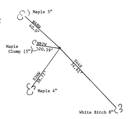
4" x 3' Iron Pipe 4" diameter brass cap
