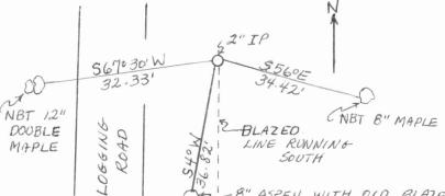
I SET A NEW 2" BLACK IRON PIPE WITH A MARKED BRASS CAP. STONES PLACED AROUND PIPE.
